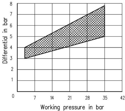
DIFFERENTIAL PRESSURE OF IPNB-80 PRESSURE SWITCH
