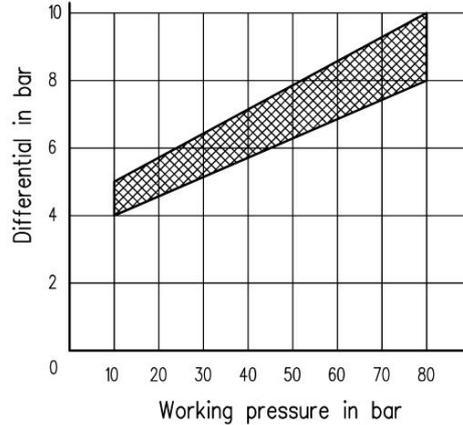
DIFFERENTIAL PRESSURE OF IPNB-160 PRESSURE SWITCH
