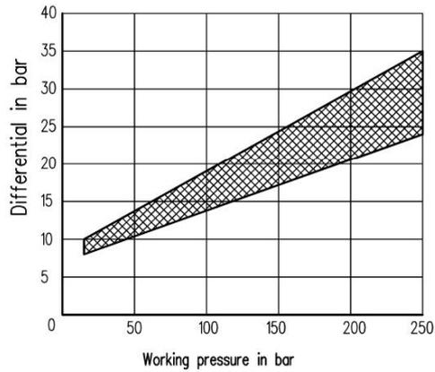
DIFFERENTIAL PRESSURE OF IPNB-350 PRESSURE SWITCH
