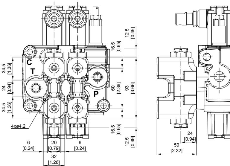
**BSP1 Kit:** Block with valve on port A
