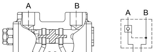
**BSP2 Kit:** Block with valve on port B
