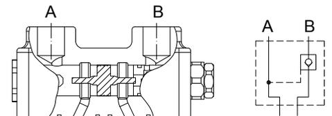
**BSP3 Kit:** Block with valve on port A and B
