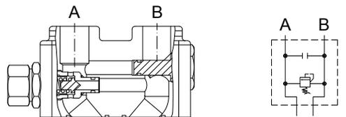
**P3 Kit:** Block with valve on port A and B
