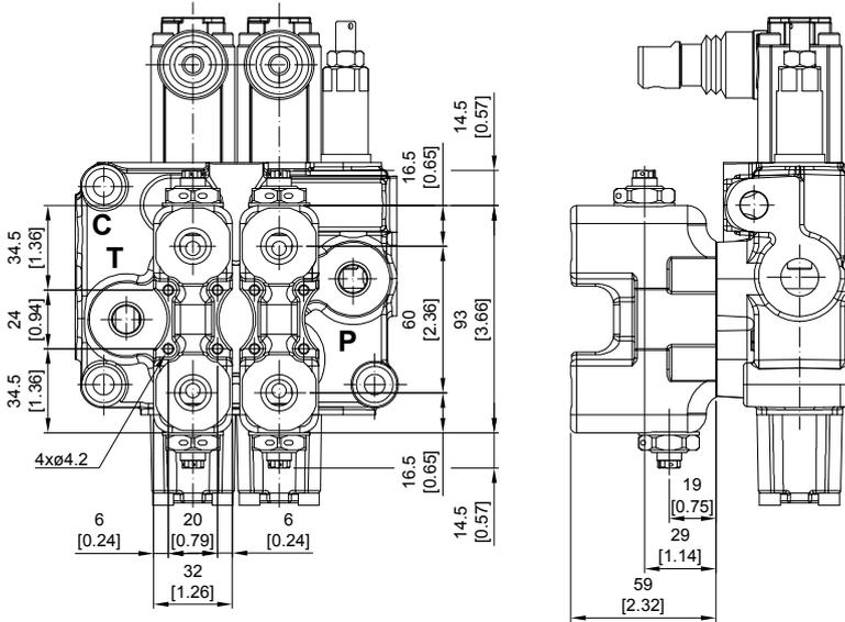
**P1 Kit:** Block with valve on port A
