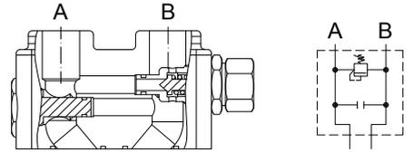
**P2 Kit:** Block with valve on port B
