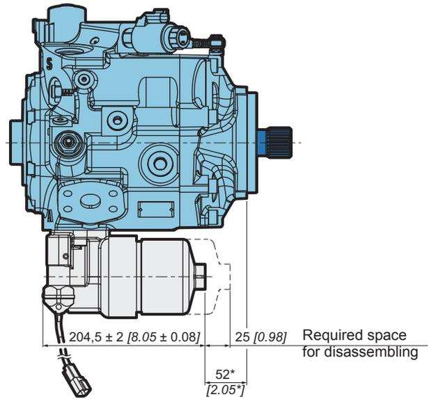
\* 38 [1.50] for 2-bolt bearing flange (option M)
