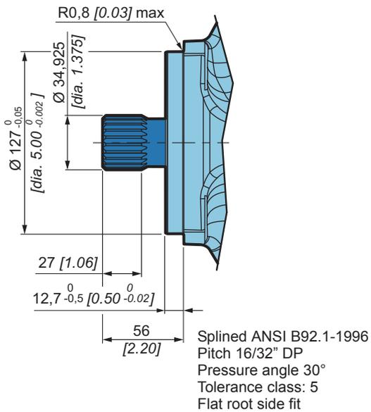
**3** 23 teeth; Shaft torque: 1000 Nm [8 851 in.lbf] (without radial force)
