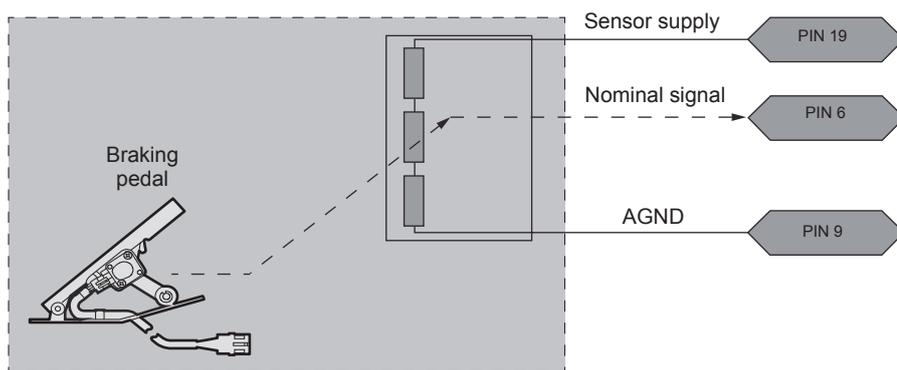
Safety requirements for compliance PLd, the braking pedal must:
