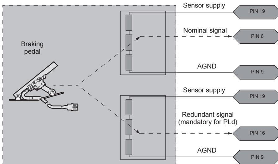
Safety requirements for compliance PLd, the braking pedal must:
