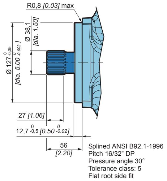
**5** 13 teeth; Shaft torque: 1500 Nm [13 276 in.lbf] (without radial force)
