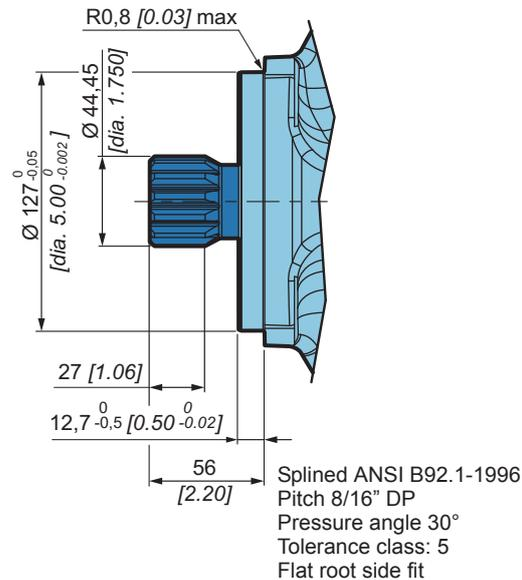
**6** 14 teeth; Shaft torque: 600 Nm [5 310 in.lbf] (without radial force)
