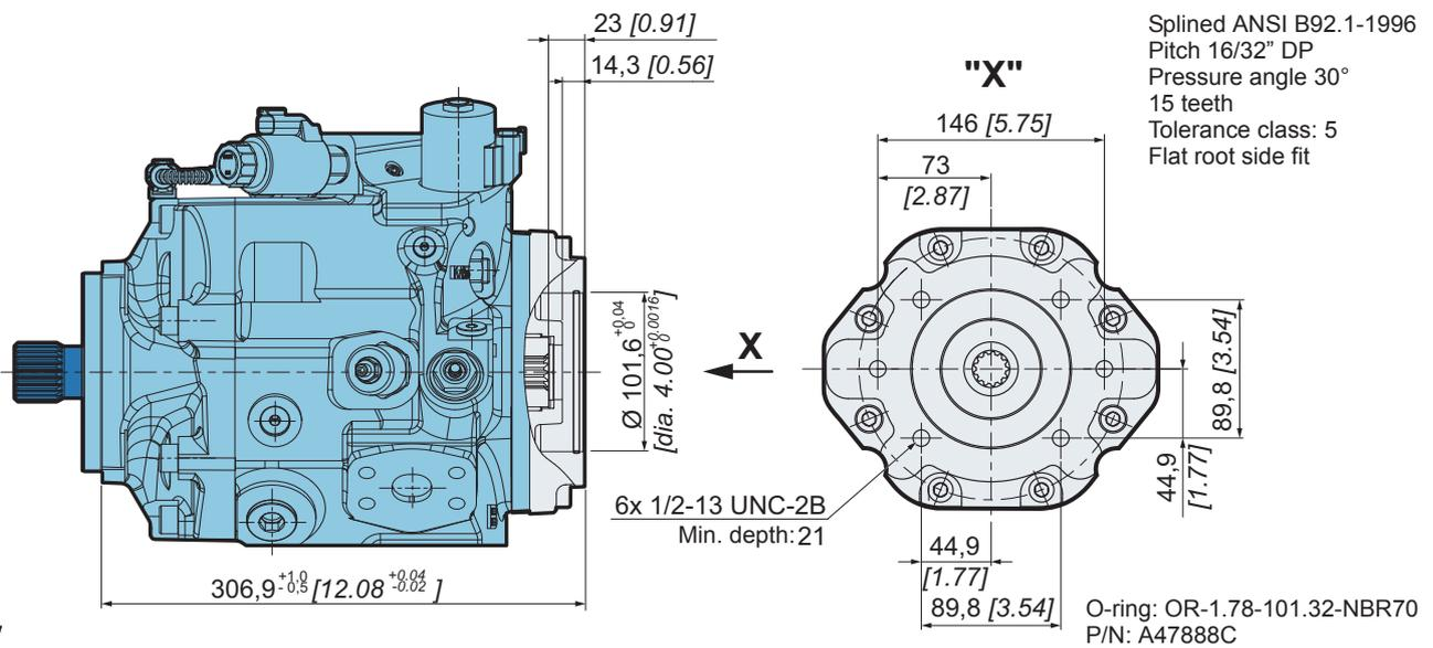
4 SAE-C; Coupling torque: 701 Nm [6204 in.lbf]; minimum active spline length: 14,5 mm [0.57 inch]
