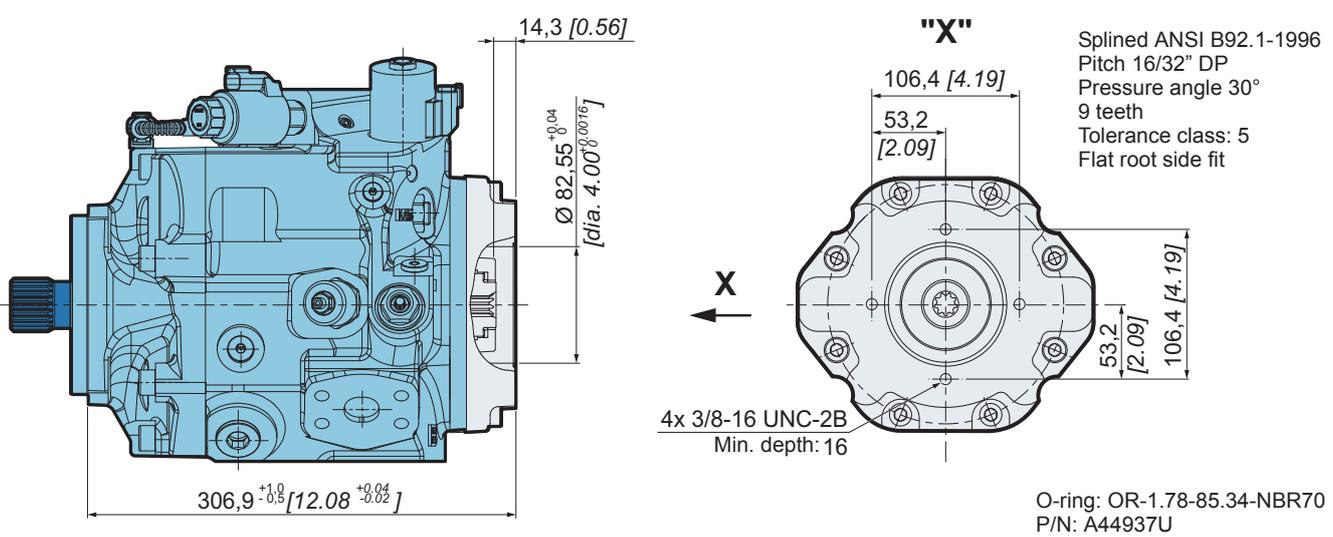
**2 SAE-B; Coupling torque: 283 Nm [2505 in.lbf]; minimum active spline length: 12 mm [0.47 inch]**
