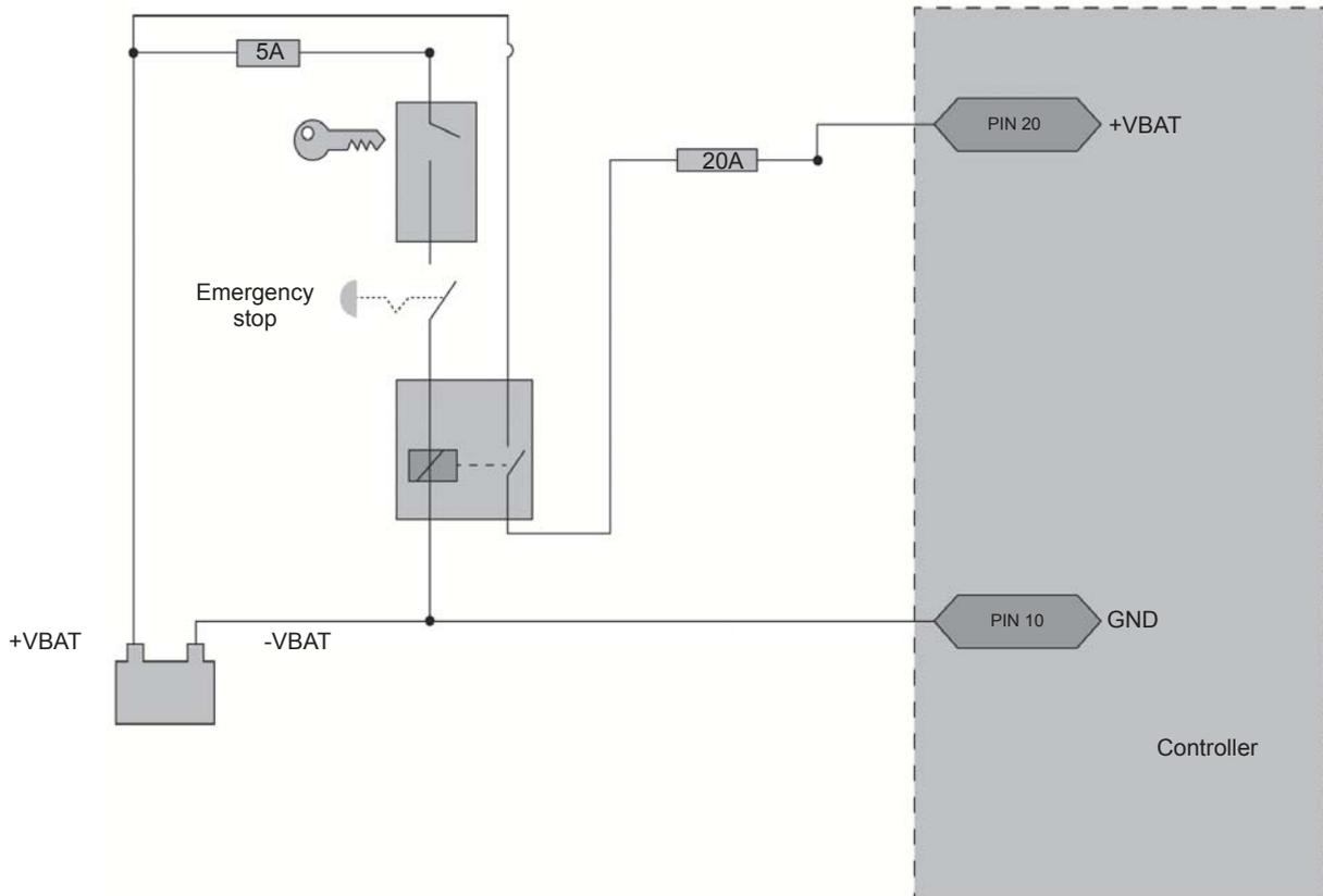
The correct wiring of the power supply pin (+VBAT) and pin connected to ground, is shown in previous figure. Power supply must be connected through an automotive fuse SAE J1284 20A.
