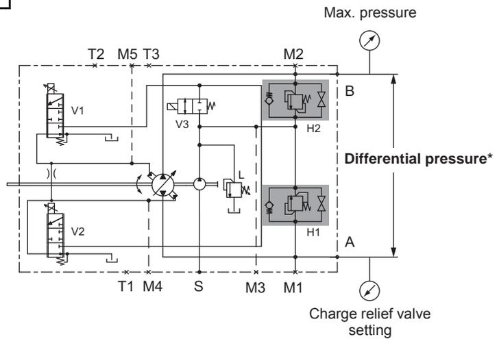
\* Differential pressure = High pressure relief valve setting
