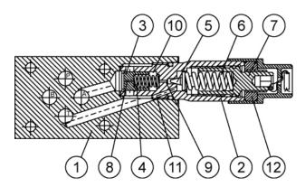
Pilot operated pressure relief valves type VP-RT of sandwich plate design, for vertical stacking, are used for maintaining and limiting the maximum pressure in a hydraulic system.
