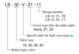
★ Use high-vent pressure types if the shifting time from unloading to on-loading is reduced.
