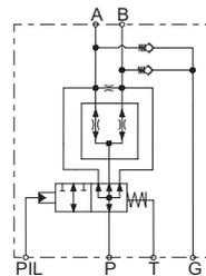
Hydraulic by-pass control with charge check and relief valves.
