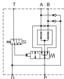
Electric by-pass control with charge check and relief valves.
