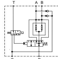
Electric by-pass control with charge check valves.
