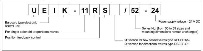
The UEIK-11RS\*/52 card is an electronic control unit Eurocard type for closed loop control of single solenoid proportional valves with positional feedback control.
