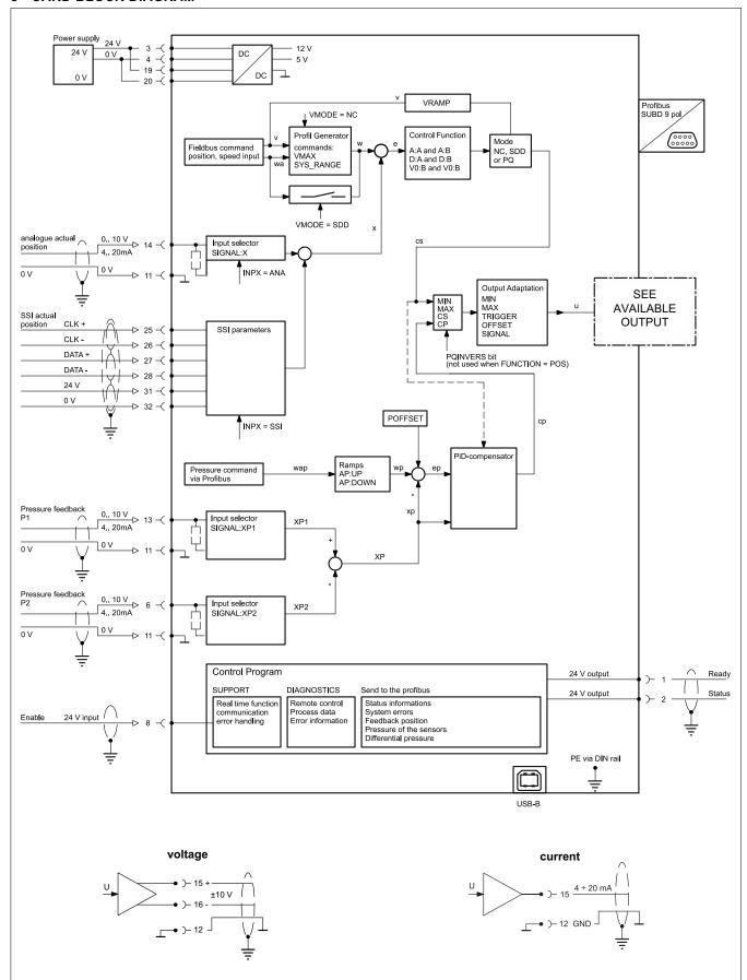
**NOTE**: If the card is configured as simple positioning control without pressure limitation then the output value is calculated just from the output of the position controller (CS) instead of apply MIN and MAX parameters. MIN/MAX are selected by the PQINVERS bit (Profibus).
