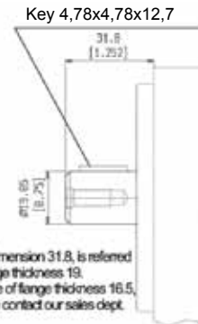
code 85 Max torque 130 Nm (1151 lbf in) 3/4" SAE A parallel
